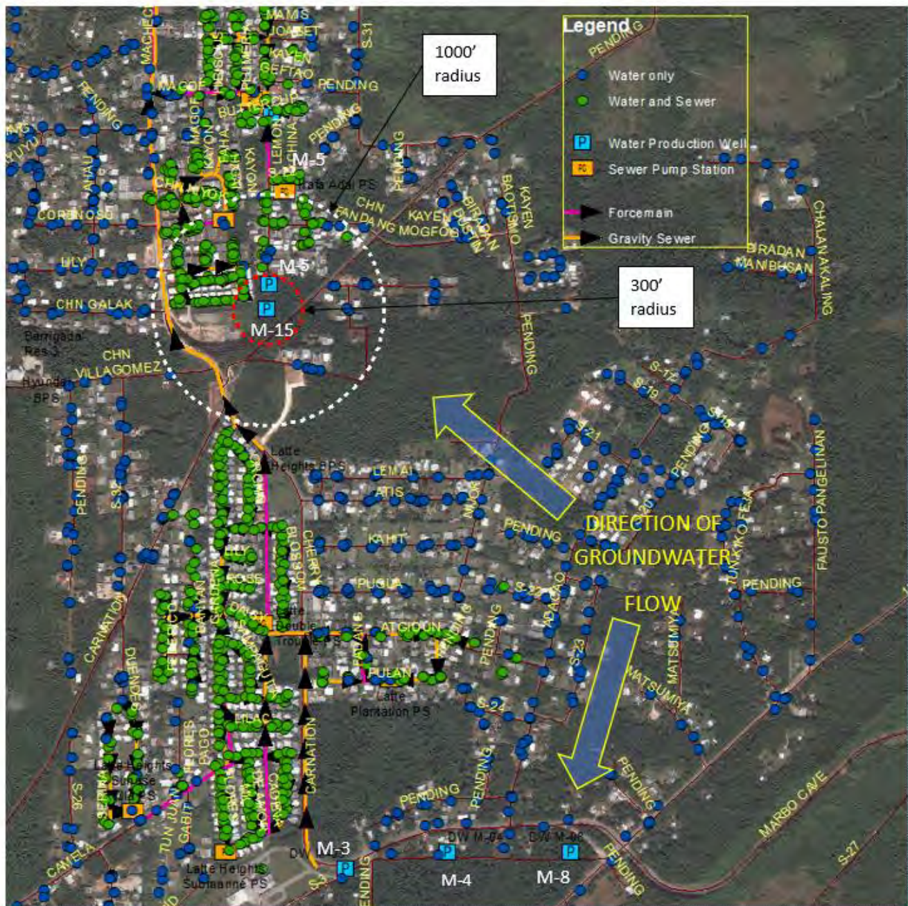
Figure B3. Well M-15's high concentration levels may be attributed to unsewered areas to the southeast. Sewer mains will be extended and water customers will be notified of their requirement to connect to the sewer system. Housing area to the north will be smoke tested for customers that are connected but not paying for sewer service.
