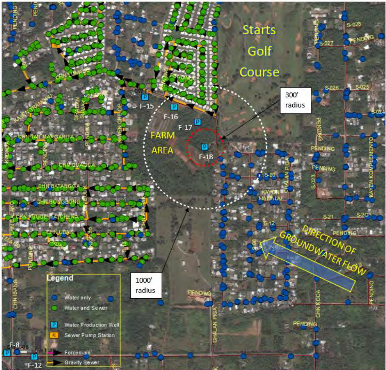
Figure B2. Well F-18 is bordered by a golf course, farmland, and a housing subdivision to the southeast comprising of water customers with no sewer connection. GWA will coordinate with GEPA and Department of Agriculture to investigate the farm area for land use compliance concerning groundwater protection. Sewer mains will need to be extended southeast and water customers will be notified of their requirement to connect to the sewer system. Moreover, the subdivision is upgradient hydro-geologically to wells F-18, F-17, F-16, and F-15.
